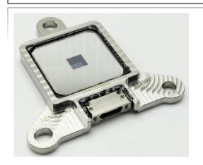
Radiation hardened fine Sunsensor for nano-satellite applications.
